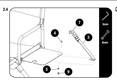
Secure the Strap (Item 3) to the Table Top (Item 1) using M5 x 10 Button Head screw  $\,$ (Item 4) and Nyloc Nut (Item 5). Place the Table Hook (Item 7) over the arm rest and adjust the Strap (Item 3) until the Table Top (Item 1) is level.
