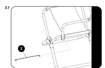
Slide the Table Hinge (Item 2) in between the tube and the chair material as shown.
