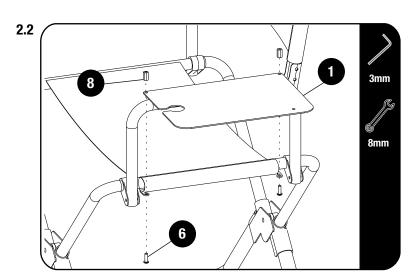
Asemble the Table Top (Item 1) to the Table Hinge (Item 2) using M5 x 15 Button Head screws and Long Hex Nuts (Item 8)
